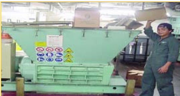
Cruise ships are equipped with numerous waste processing machines, such as this shredder that minimizes trash.
